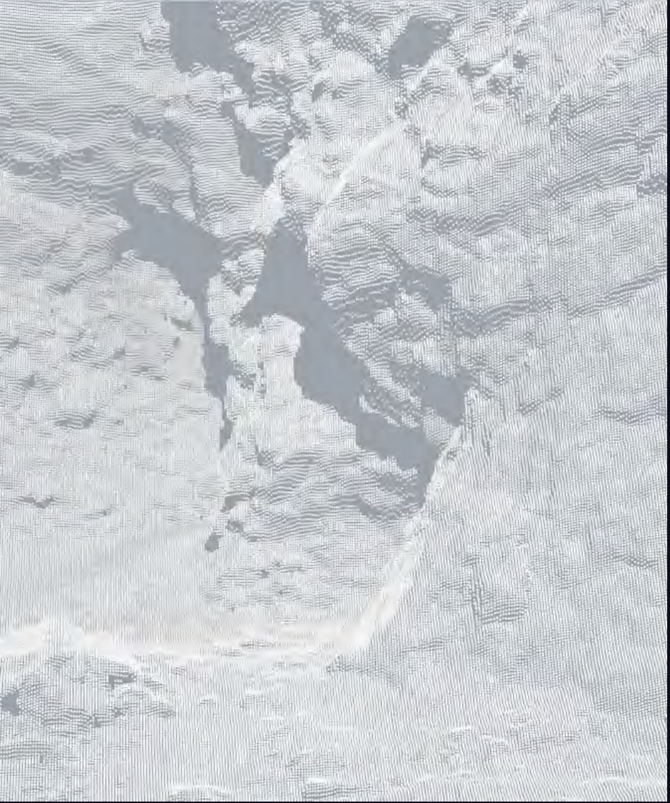
Different stages of reconstruction of a scan of the Balme cave, going from the cloud of points to a complete mesh.
