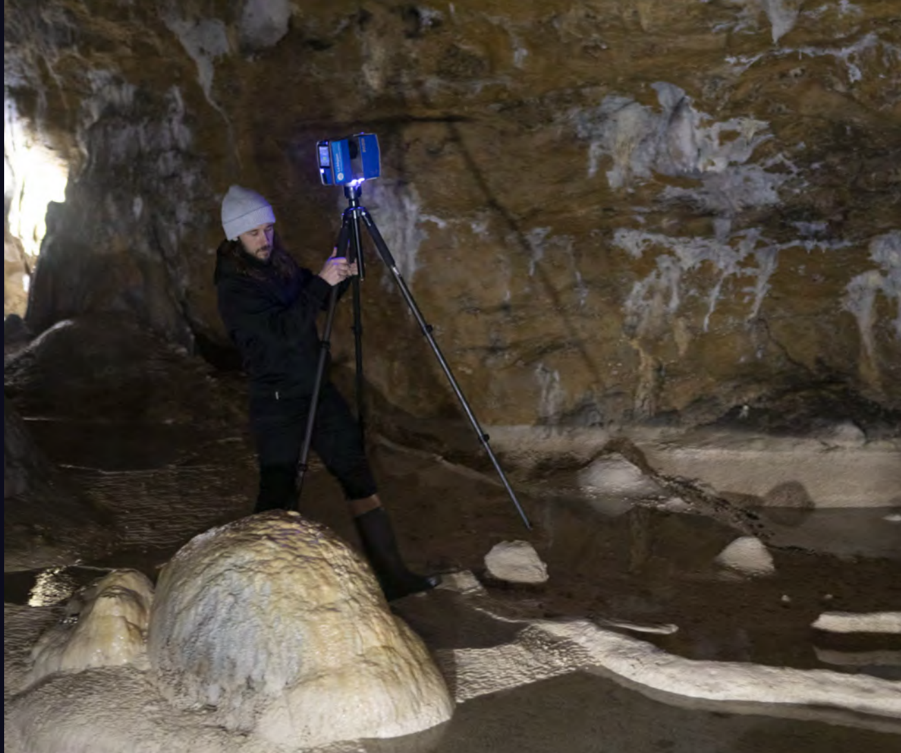
Use of Scan Faro by an INSA technician, Grotte de la Balme, March 2022
